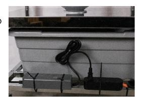
38. Plug the Plug Adapter into the Power Supply
